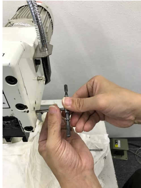
16. Tap on the holes.
